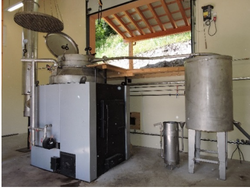
Steam distillation, l'Essencier, Icogne
