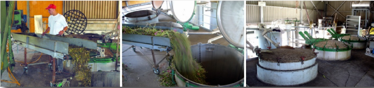
Steam distillation, distillerie de Bassins sarl
